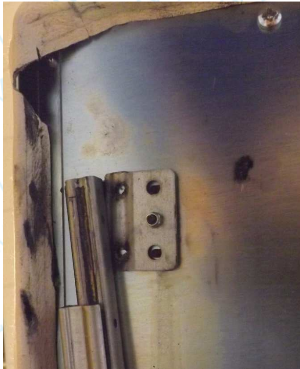
Picture 11: Leg rest runner fixing damage of the 'Cowe-Kebe-Electric Chair'
