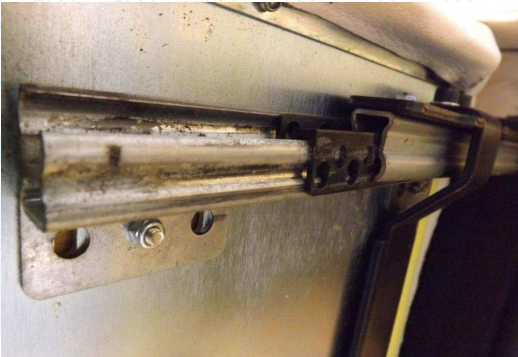
Picture 5: Leg rest runner damage of the 'Cowe-Kebe-Electric Chair'
