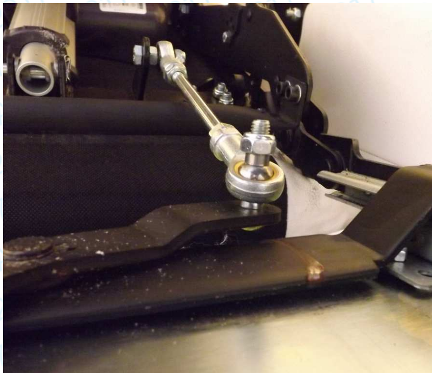
Picture 13: Leg rest crossrail damage of the 'Cowe-Kebe-Electric Chair'
