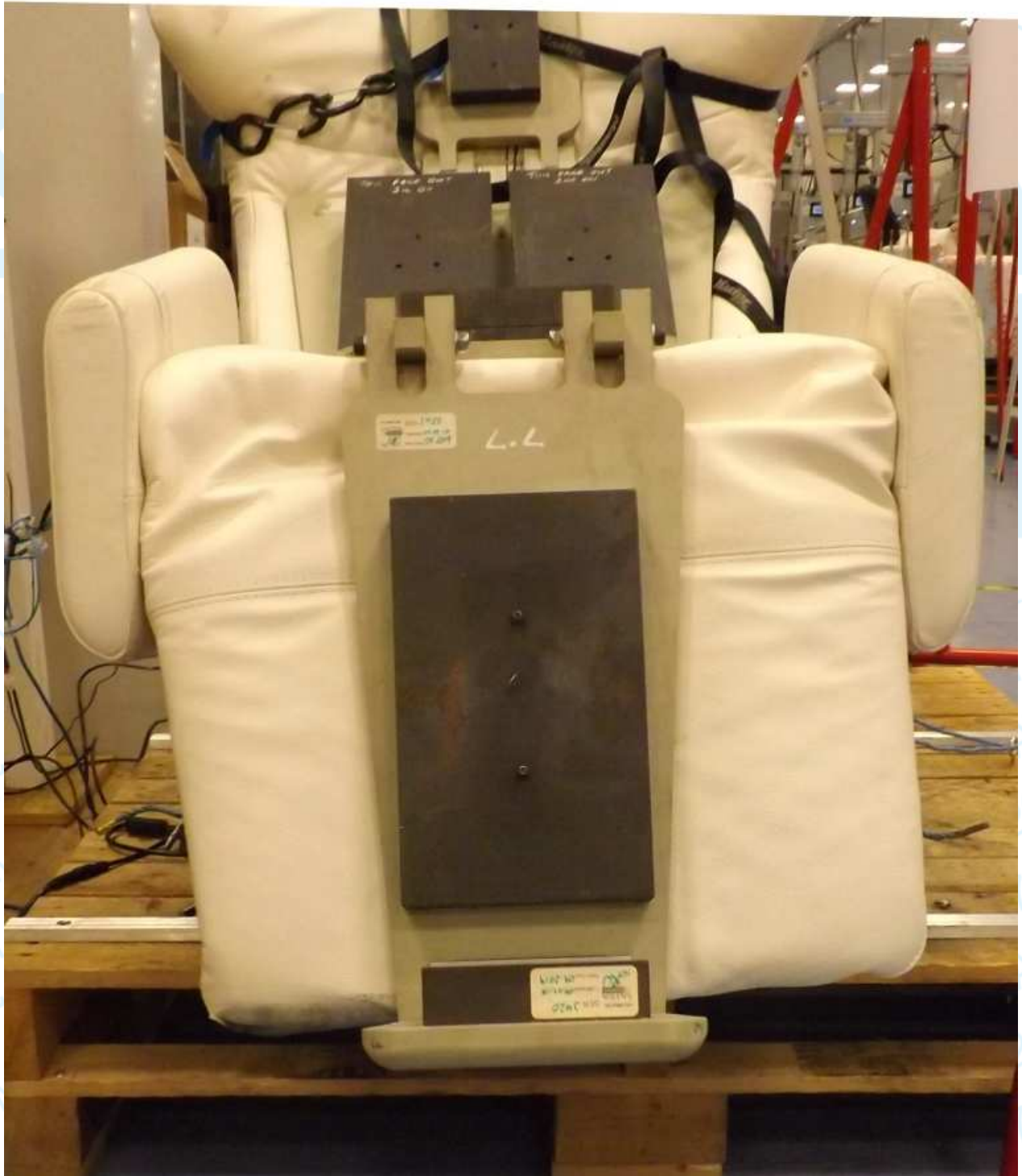
Picture 9: Leg rest misalignment of the 'Cowe-Kebe-Electric Chair'
