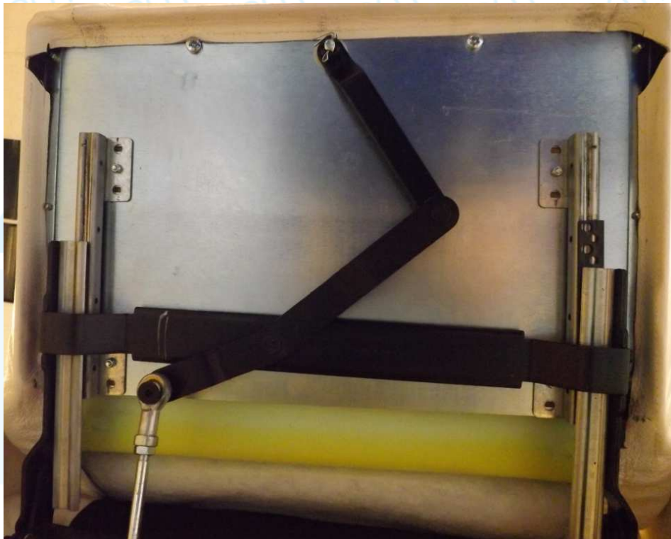
Picture 7: Leg rest misalignment of the 'Cowe-Kebe-Electric Chair'
