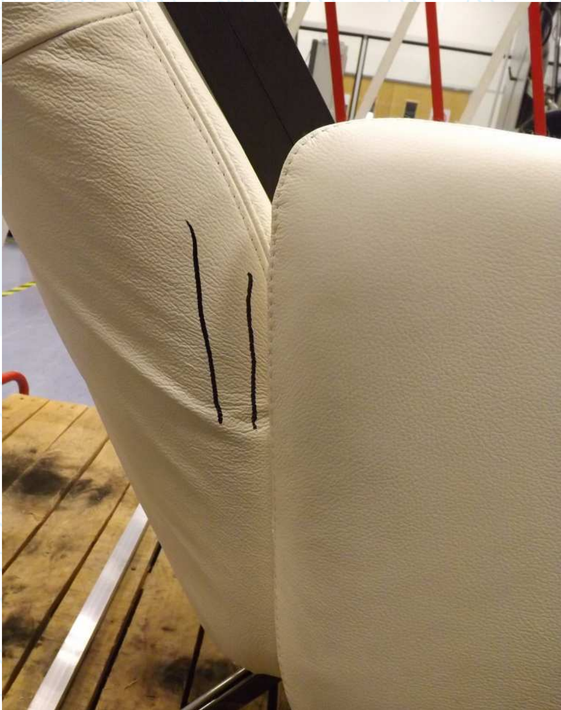
Picture 14: Back rest wear of the 'Cowe-Kebe-Electric Chair'
