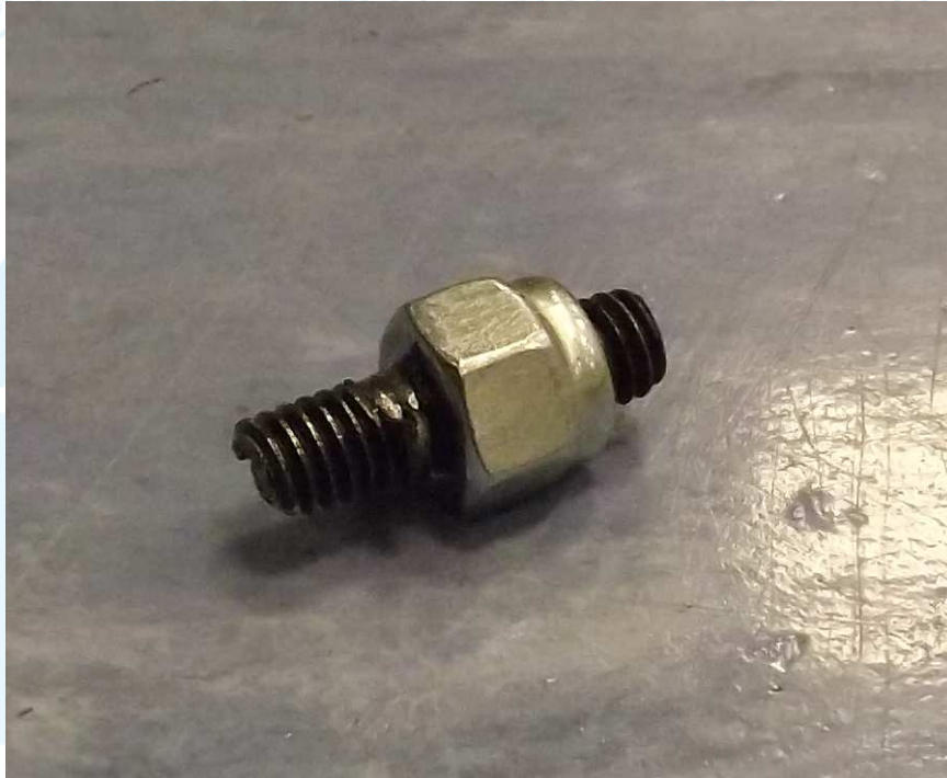
Picture 12: Leg rest runner fixing damage of the 'Cowe-Kebe-Electric Chair'
